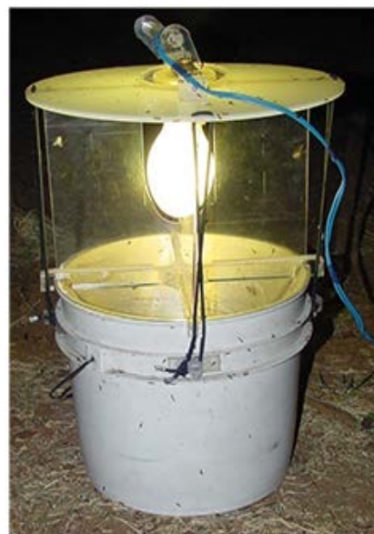
Photo 1. Portable light trap
